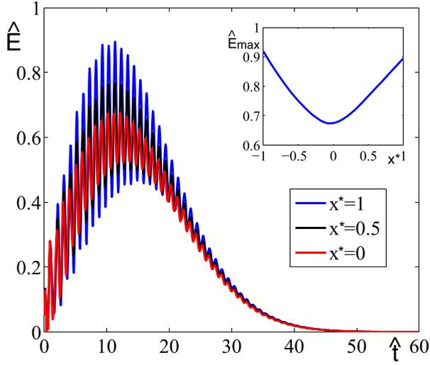
FIG. 7. Dependence of  $\hat{E}$  on  $x^*$  for  $\hat{\omega} = 2\pi$ ,  $\hat{k} = 0.25$ ,  $\mu = 0.05$ ,  $\beta^* = 0.05$ . Inset: Maximum of the electric field  $\hat{E}_{max}$  as a function of position  $x^*$ .
