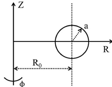
FIG. 1. Magnetic field geometry:  $a$  and  $R_0$  are the minor and the major radii of a torus.
