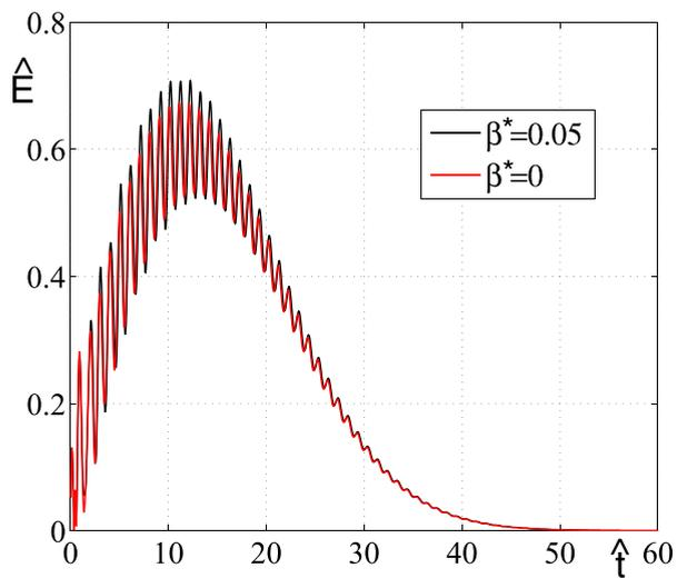
FIG. 2. Influence of the inhomogeneity of the magnetic field on the transient growth for  $\hat{\omega} = 2\pi$ ,  $\hat{k} = 0.25$ ,  $\mu = 0.05$ ,  $x^* = 0.25$ .
