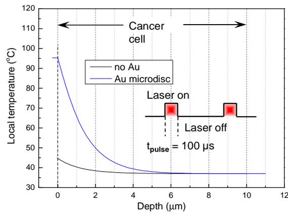
**FIG. S2.** COMSOL Multiphysics simulation model of a GaN NM attached to a cell while being heated by a laser beam. Temperature depth profile for the case when the NM is in direct contact with the cell and when an Au microdisc is inserted. The laser beam was pulsed at a 100  $\mu$ s long excitation pulse. Ambient temperature was taken as 37°C in these simulations.
