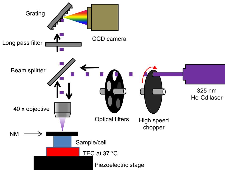
**FIG. S3.** Experimental setup used to measure thermal diffusivities. Schematic diagram depicting the beam optical path for the excitation 325 nm laser as well as the PL emission from the NMs.
