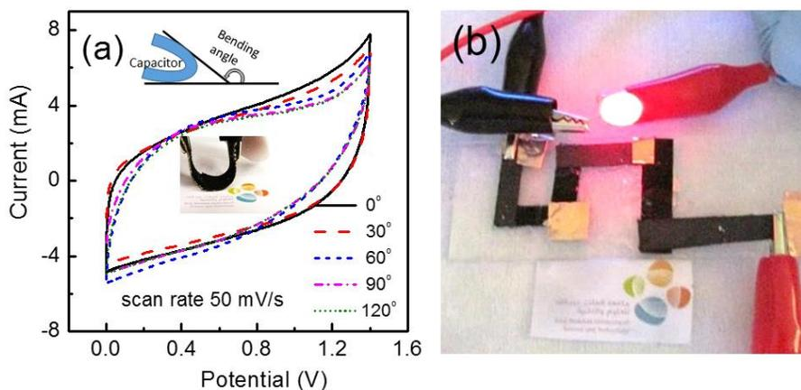
(a) CVs of solid state device measured at different angles (inset shows the schematic for the measurement of the bending angles and the optical image of the flexible supercapacitor device). (b) Optical images displaying lighting up of an LED using three flexible supercapacitors connected in series.
