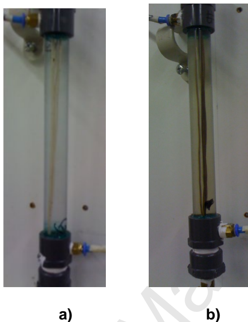
5 Fig. 12 Fouling layer developed on HFFO lumen fiber module used for a) AL-FS and b) 6 AL-DS respectively
