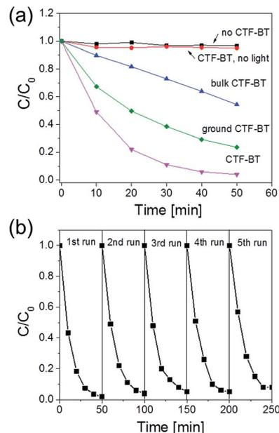
Fig. 3 (a) Photoreduction rates of 4-NP to 4-AP using hollow CTF-BT as photocatalyst with control experiments. Reaction conditions: CTF-BT (5 mg), 2 mM 4-NP (1 ml), NaBH<sub>4</sub> (10 mg), 1 M NaOH (10 μl), H<sub>2</sub>O/EtOH (3 : 1) 4 ml, white LED lamp ( $\lambda > 420$  nm). (b) Repeating experiments of photoreduction of 4-NP.
