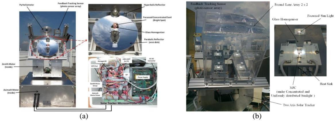
Figure 1 (a) Developed CPV system; (b) Cassegrain mini dish with fresnel lens
