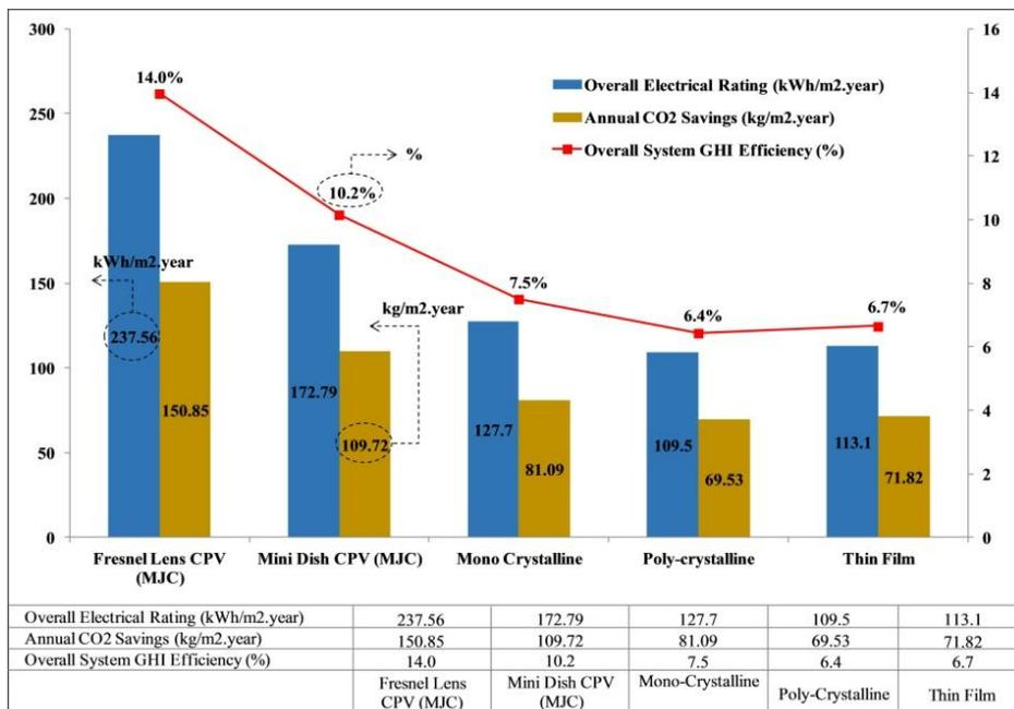
Figure 3 Overall Electrical Rating of CPV Systems Compared to Other Photovoltaic Systems and CO<sub>2</sub> Savings
