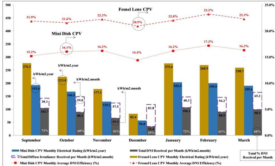
Figure 2 Monthly electrical rating and monthly average efficiency of CPV systems with the DNI received
