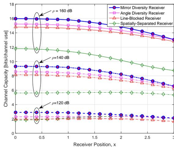
Fig. 2. Channel capacity as a function of the receiver position in SSR, LBR, ADR, and the proposed MDR for different SNRs.
