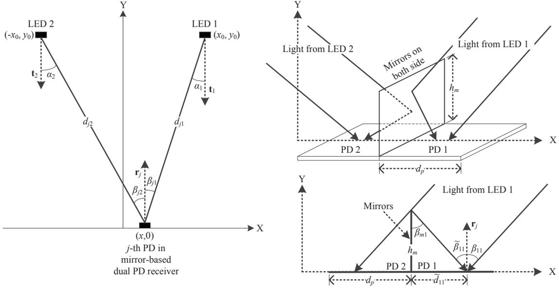
Fig. 1. System model of a 2-dimensional  $2 \times 2$  OWC-MIMO link equipped with the proposed mirror diversity receiver; The geometry of transmitter-receiver pair (left), the structure of proposed MDR (top right), and the example for its reception of incident light from the 1st LED with  $\mathbf{r}_j = [0 \ 1]^T$  (bottom right).
