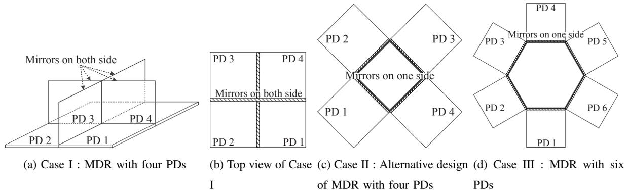
Fig. 4. Generalization of the proposed MDR with multiple PDs. Hatching lines in the figure symbolize a mirror.
