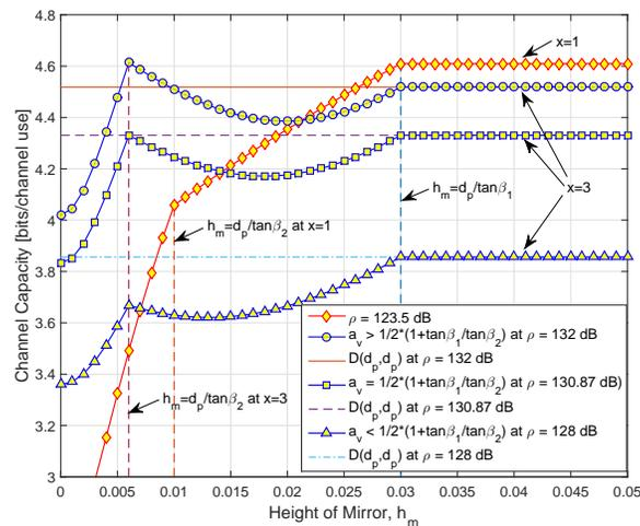
Fig. 3. Channel capacity of the proposed MDR as a function of height of perfect mirror at the receiver positions,  $x = 1$  and  $x = 3$ , for different SNRs.
