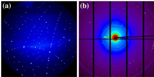
**Fig. 9** a Laue diffraction pattern of a crystalline phase found in type F fly ash obtained with polychromatic (*white*) beam radiation b Debye-Scherrer diffraction pattern from a HVFA paste microstructure obtained with monochromatic beam radiation.
