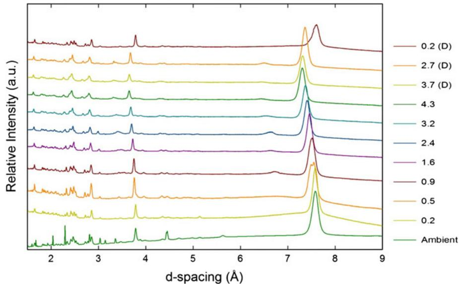
**Fig. 11** Integrated X-ray diffraction patterns of monocarboaluminate with different pressures. The *numbers* indicate applied hydrostatic pressures (GPa). The top three patterns (D) were collected during decompression (Moon et al. 2012).
