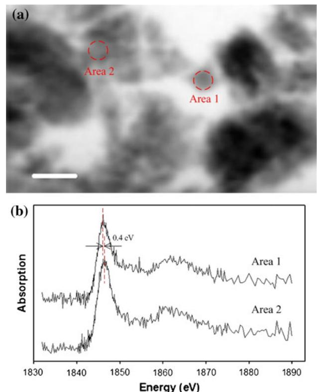
**Fig. 6** a STXM image of the Al-substituted C-S-H phase: the scale bar is 1  $\mu\text{m}$ . b Si K-edge XANES spectra of the corresponding areas in (a).
