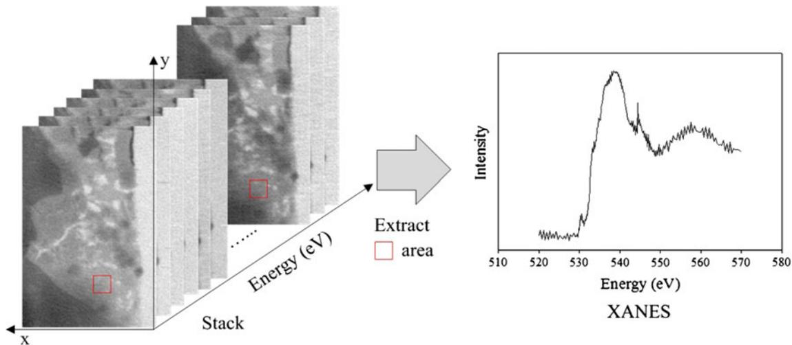
**Fig. 4** XANES extraction from the stack, a collection of single images at incremental energy levels.
