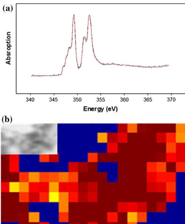
Fig. 8 a XANES spectrum of Ca L<sub>III,II</sub>-edge obtained from the C3A hydration product: *solid lines* are the experimental XANES spectrum, and the *dashed line* is the modeled spectrum based on LC fitting b Contour map of the C3A hydration product showing the monosulfate distribution based on the LC fitting result.
