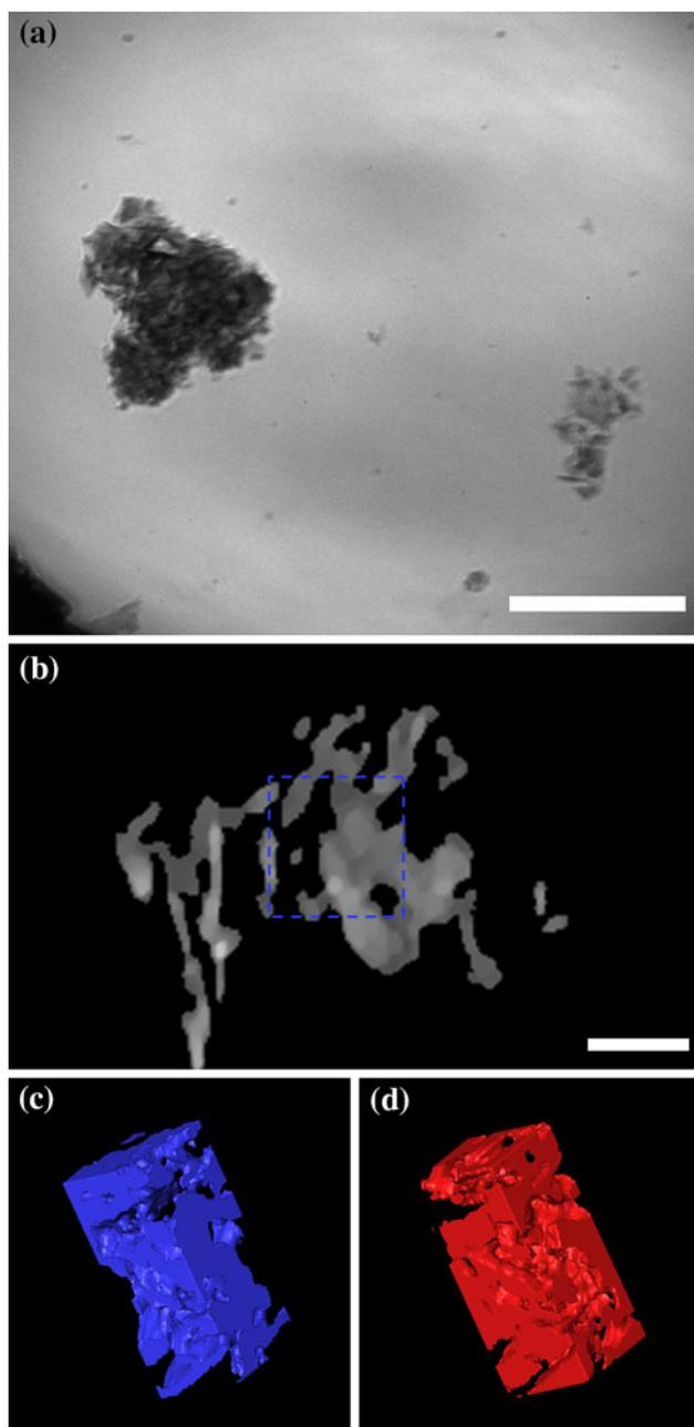
**Fig. 1** Soft TXM nCT taken at 510 eV incident X-ray. Typical TXM image is shown in (a), with a  $3\ \mu\text{m}$  scale bar. A reconstructed tomogram of a particle  $\sim 5\ \mu\text{m}$  width is shown in (b), with a  $1\ \mu\text{m}$  scale bar. A 3-D reconstruction of a  $1.5 \times 1.5 \times 5\ \mu\text{m}$  section (and shown in dotted line in (b)) is shown in (c). Its negative imprint, or the voids, is shown in (d).
