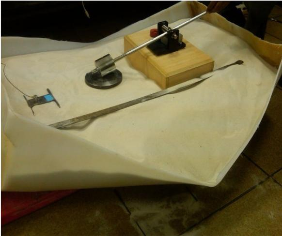
**Figure 1: A picture of a container of Sand that includes the streamer to the left and the source to the right.**
