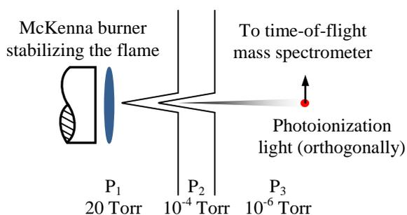
Figure 1. Schematic diagram describe the experimental setup.
