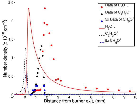
Figure 5: Distribution of positive ions across the flame in comparison with experiment.
