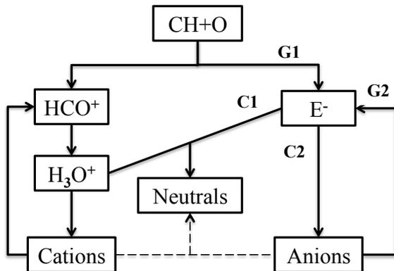
Figure 2: Flowchart of ion chemistry. G1 and G2 are the channels generating  $\text{E}^-$ . C1 and C2 are the channels consuming  $\text{E}^-$ .
