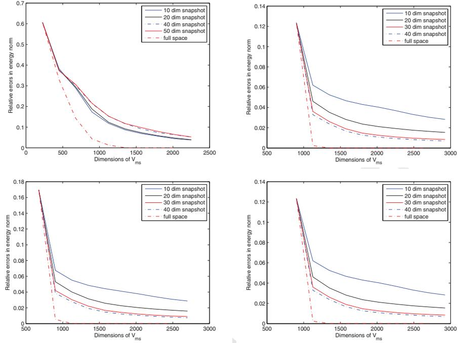
Figure 6: Performance comparison for the use of reduced dimensional space for online basis construction for the permeability field in Figure 2. Top-Left: One basis. Top-Right: Two basis. Bottom-Left: Three basis. Bottom-Right: Four basis.
