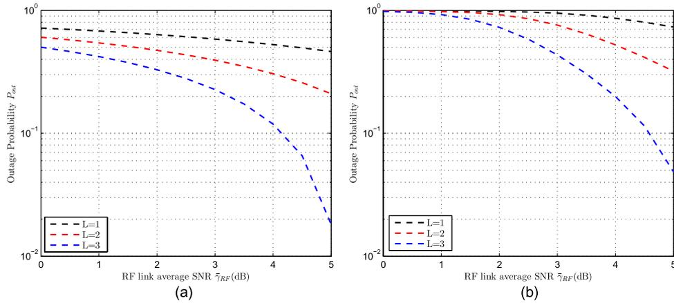
Fig. 3. Outage probability of hybrid FSO/RF system with power adaptation as a function of the average SNR of the RF link considering IM/DD FSO detection technique, with  $\gamma_T = 10$  dB, weak atmospheric turbulence ( $\alpha = 2.902$ , and  $\beta = 2.51$ ),  $\bar{\gamma}_{FSO_2} = 0$  dB,  $\xi = 1$ , and Nakagami parameter  $m = 2$ . (a) Using  $\gamma_{RF}$ -based TCI. (b) Using  $\gamma_{RF} + \gamma_{FSO}$ -based TCI.
