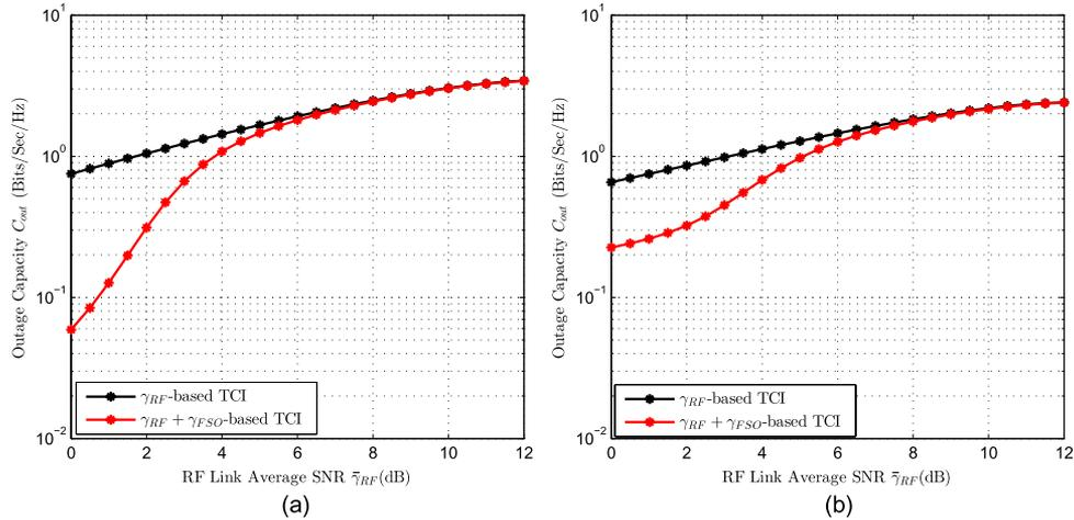
Fig. 5. Outage capacity of hybrid FSO/RF system with power adaptation as a function of the average SNR of the RF link with  $\gamma_T = 10$  dB, weak atmospheric turbulence ( $\alpha = 2.902$ , and  $\beta = 2.51$ ),  $\gamma_{FSO} = 0$  dB,  $\xi = 1$ , and Nakagami parameter  $m = 2$ . (a) Using heterodyne detection technique with FSO link ( $r = 1$ ). (b) Using IM/DD detection technique with FSO link ( $r = 2$ ).
