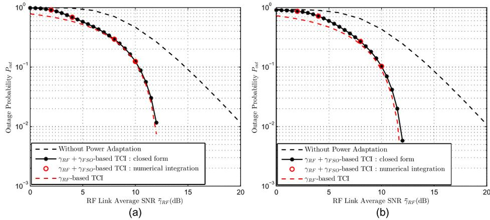
Fig. 1. Outage probability of hybrid FSO/RF system with and without power adaptation as a function of the average SNR of the RF link with  $\gamma_T = 10$  dB, weak atmospheric turbulence ( $\alpha = 2.902$ , and  $\beta = 2.51$ ),  $\bar{\gamma}_{FSO} = 0$  dB,  $\xi = 1$ , and Nakagami parameter  $m = 2$ . (a) Using heterodyne detection technique with FSO link ( $r = 1$ ). (b) Using IM/DD detection technique with FSO link ( $r = 2$ ).
