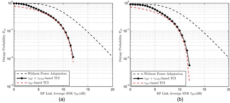
Fig. 4. Outage probability of hybrid FSO/RF system with and without power adaptation as a function of the average SNR of the RF link with  $\gamma_T = 10$  dB, strong atmospheric turbulence ( $\alpha = 2.064$ , and  $\beta = 1.342$ ),  $\bar{\gamma}_{FSO_2} = 0$  dB,  $\xi = 4$ , and Nakagami parameter  $m = 2$ . (a) Using heterodyne detection technique with FSO link ( $r = 1$ ). (b) Using IM/DD detection technique with FSO link ( $r = 2$ ).
