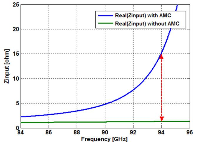
Fig.3. Input impedance of the dipole with and without AMC.
