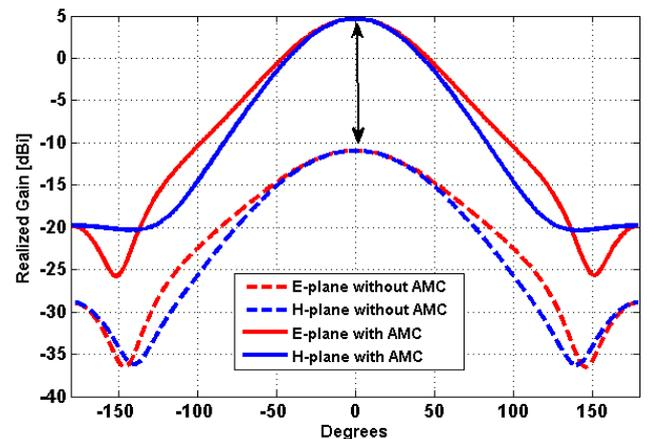
Fig. 4. Realized gain of the dipole antenna with (solid lines) and without (dashed lines) AMC in the E-plane and H-planes.
