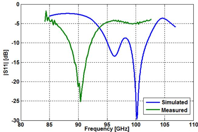
Fig. 6. Measured and simulated reflection coefficient
