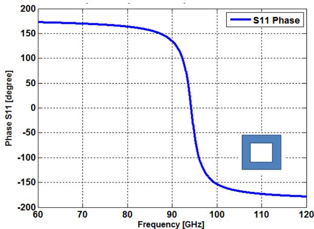
Fig. 2. In-phase response of the proposed AMC.
