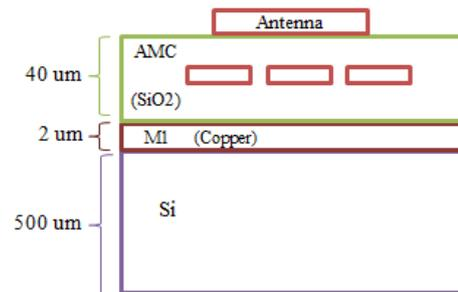
Fig.1. Lateral view of the considered CMOS compatible stack up.
