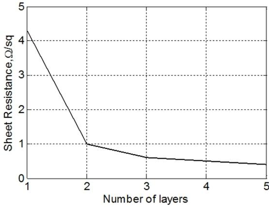
Fig. 4: Sheet resistance of the printed metal.
