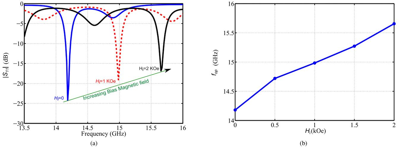
Fig. 2: Simulated frequency-tuning of the slotted waveguide antenna. (a) Reflection Coefficient. (b) Operating frequency versus bias field.
