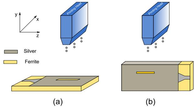
Fig. 1: Inkjet Printing of a rectangular waveguide. (a) Top metalization pattern. (b) Side metalization pattern.
