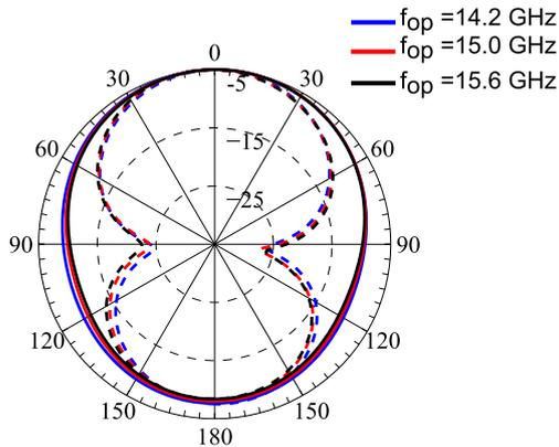
Fig. 3: Radiation pattern at at different operating frequencies, E-plane (solid-lines) and H-plane (dashed-lines).
