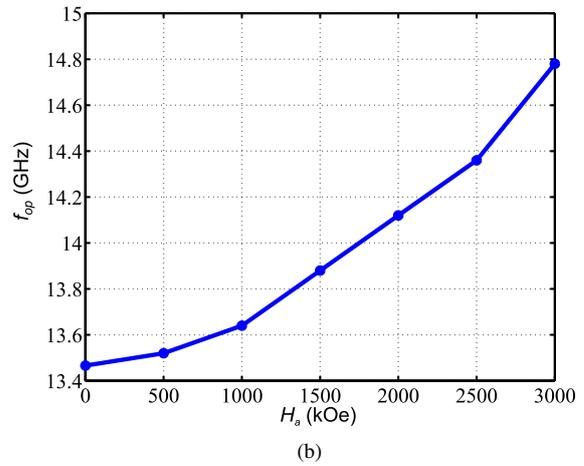
Fig. 6: Measured frequency-tuning of the slotted waveguide antenna. (a) Reflection Coefficient. (b) Operating frequency versus bias field.
