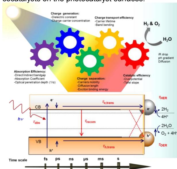
Fig. 1. Conceptual scheme for photocatalytic OWS reaction.
