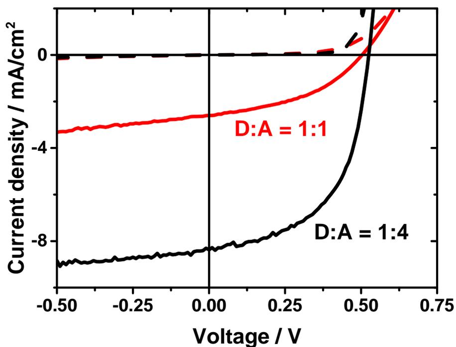
*Figure S1.* Current-Voltage (J-V) characteristics of pBTTT:PC<sub>70</sub>BM solar cells at a donor-acceptor ratio of 1:1 (solid red line) and 1:4 (solid black line) and respective dark currents (dashed lines).
