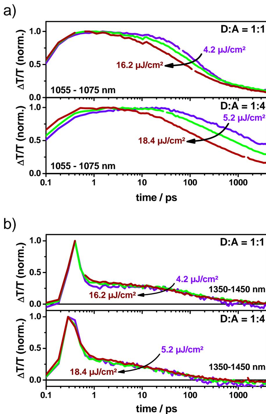
Figure S3. (a) Intensity-dependence of the dynamics of the charge-induced absorption in the spectral range from 1055-1075 nm of a pBTTT:PC<sub>70</sub>BM blend at ratios of 1:1 (upper panel) and 1:4 (lower panel). (b) Dynamics tracked between 1350-1450 nm, that is the spectral range, in which the pBTTT exciton-induced and charge-induced absorption occur. Note the fast sub-ps signal decay indicating ultrafast polymer exciton dissociation in both blends.
