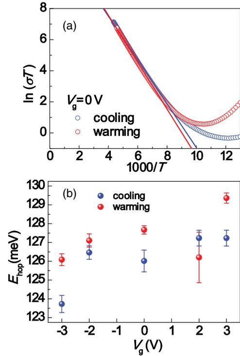
FIG. 3. (Color online) (a) Small polaron fitting to the high-temperature transport data for both the warming and the cooling processes. For clarity, only the zero gate data are shown. (b) Plot of the activation energy  $E_{\text{hop}}$  as calculated from the fitting to the small polaron model versus the gate voltage.
