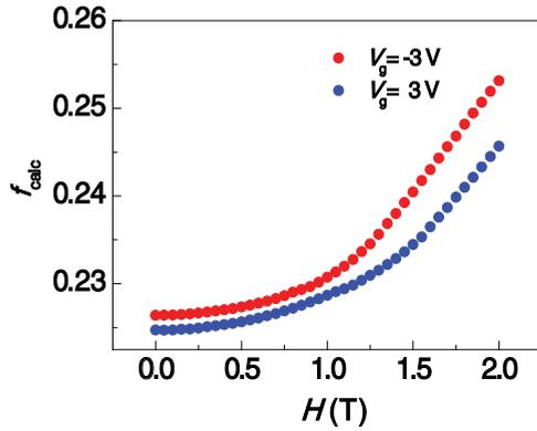
FIG. 7. (Color online) Fraction of the FM phase vs the magnetic field at 80 K for gate voltages of +3 and -3 V as estimated from the GEM theory.
