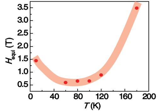
FIG. 8. (Color online) Plot of equivalent magnetic field  $H_{\text{equi}}$  as a function of temperature.  $H_{\text{equi}}$  represents the value of a magnetic field, which needs to be introduced on the +3 V gate biased channel in order to produce the same resistance modulation as reversing the gate bias to -3 V.
