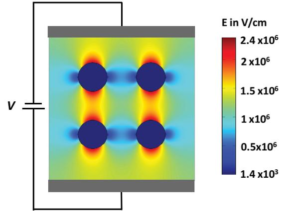
FIG. 4. (Color online) A two-dimensional toy model illustrating the local electric field distribution inside an inhomogeneous media when a voltage is applied across the electrodes. Four metallic spheres with a radius of 5 nm are embedded in an insulating host, and the total thickness of the media between the electrodes is 25 nm, which is close to the actual thickness of the PCSMO film used in our experiments.
