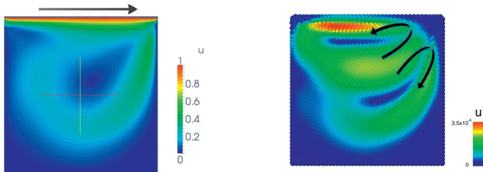
Fig. 4. Coarse (left) and fine (right) velocity profiles. SDPD fine scales are driven by the residual coarse scale. The current influence of the residual as external force, induces different vortex patterns in the simulation domain. The arrows indicate the flow direction.
