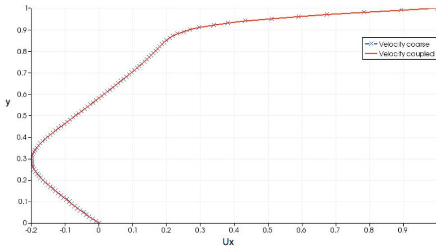
Fig. 3. Horizontal coarse-scale fluid velocity along the vertical center line for  $Re = 10^3$ . For the sake of comparison, the velocity profiles before (coarse) and after (coupled) fine scale coupling are presented.
