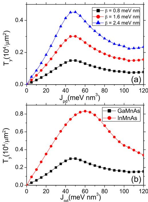
FIG. 3. The  $T_y$  component of the spin torque as a function of exchange coupling  $J_{pd}$ . (a)  $T_y$  versus  $J_{pd}$  at various values of  $\beta$ , for (Ga,Mn)As. (b)  $T_y$  versus  $J_{pd}$ , for both (Ga,Mn)As and (In,Mn)As. The magnetization is directed along the  $z$ -axis ( $\theta = 0$ ). The other parameters are the same as those in Fig. 2.
