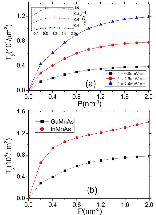
FIG. 4. The  $y$ -component of the spin torque as a function of hole concentration. (a) The  $y$ -component of the spin torque versus hole concentration at different  $\beta$ . (b) Spin torque versus hole concentration in (Ga,Mn)As and (In,Mn)As. For (Ga,Mn)As,  $J_{pd} = 55 \text{ meV nm}^3$ ; for (In,Mn)As,  $J_{pd} = 39 \text{ meV nm}^3$ . The other parameters are the same as in Fig. 3.
