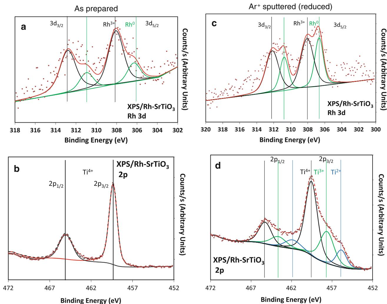
**Fig. 4** XPS Rh 3d and Ti2p of 0.5wt% Rh/SrTiO<sub>3</sub>. **a, b** As-prepared and **c, d** after Ar ions sputtering
