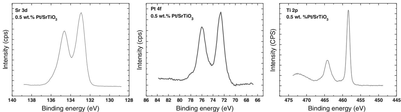
**Fig. 5** XPS Sr3d, Ti2p and Pt 4f of the as-prepared 0.5 wt% Pt/SrTiO<sub>3</sub>. The Sr to Ti atomic ratio is about 1
