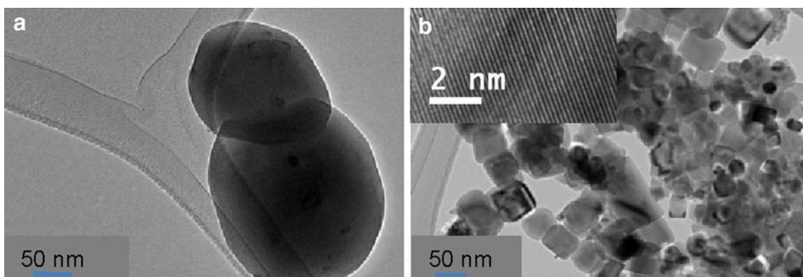
**Fig. 3** TEM of 0.5 wt% Pt/SrTiO<sub>3</sub>. **a** Commercial SrTiO<sub>3</sub> and **b** SrTiO<sub>3</sub> prepared by the sol-gel method; the inset in **b** presents the [100] cubic structure of SrTiO<sub>3</sub> evidence of a high degree of crystallinity
