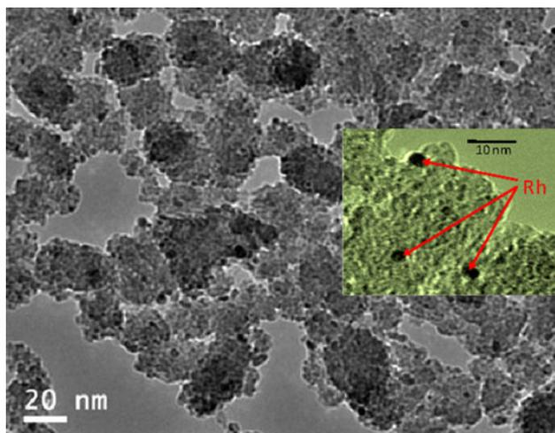
**Fig. 2** TEM of 0.5 wt% Rh/SrTiO<sub>3</sub>. Rh can be seen as dark particles in the main figure as well as the inset
