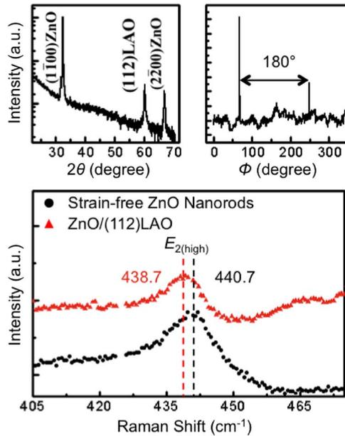
Fig. 1. X-ray diffraction pattern of (a)  $\theta$ - $2\theta$  and (b) in-plane  $\phi$  scan of ZnO film grown on (112)LAO. (c) Raman spectra of *m*-plane ZnO film grown on (112)LAO (red) and strain free ZnO nanorods (black).
