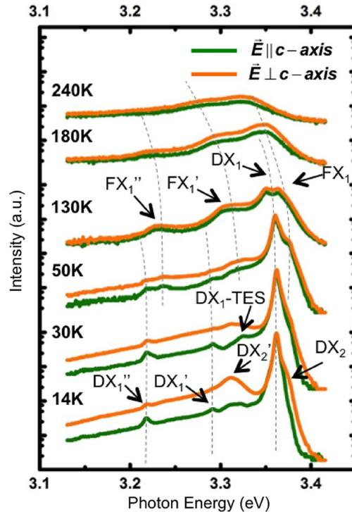
Fig. 2. Temperature dependent PL spectrum of our *m*-plane ZnO film for emission polarized in  $\vec{E} \parallel c$  (green) and  $\vec{E} \perp c$  (orange).
