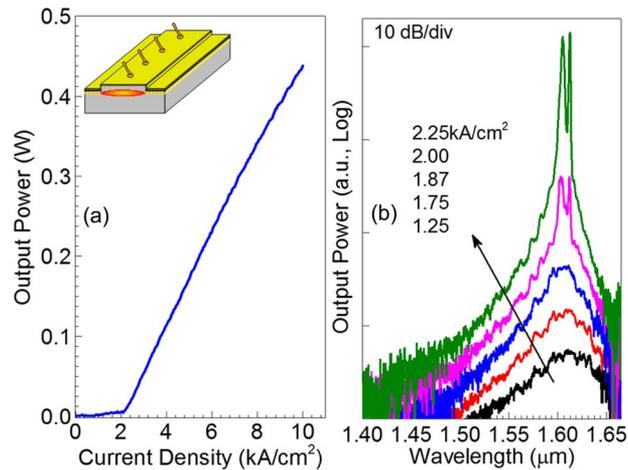
Fig. 2. Room temperature L-I characteristics of as-cleaved  $20 \times 1000 \mu\text{m}^2$  broad area Qdash laser in SP mode operation. The corresponding measured lasing spectra around the threshold current density  $J_{th} \sim 2.0 \text{ kA/cm}^2$ .
