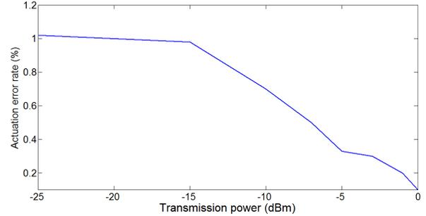
Fig. 12. Actuation error rate vs. transmission power
