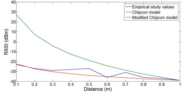
Fig. 8. Comparison between different *RSSI* (dBm) vs. Distance (m) experimental measurements and model estimation
