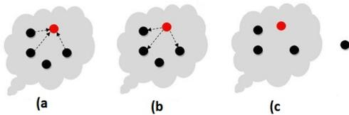
Fig. 3. a) Node does not broadcast DIS packet b) Master assumes node had left the neighborhood c) Node is removed. (Red circle denotes master, black circle denotes slave)
