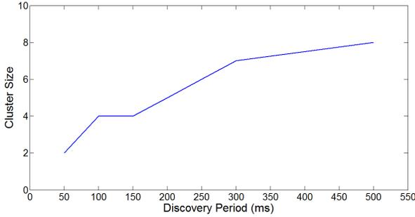
Fig. 10. Minimum discovery period vs. different cluster sizes
