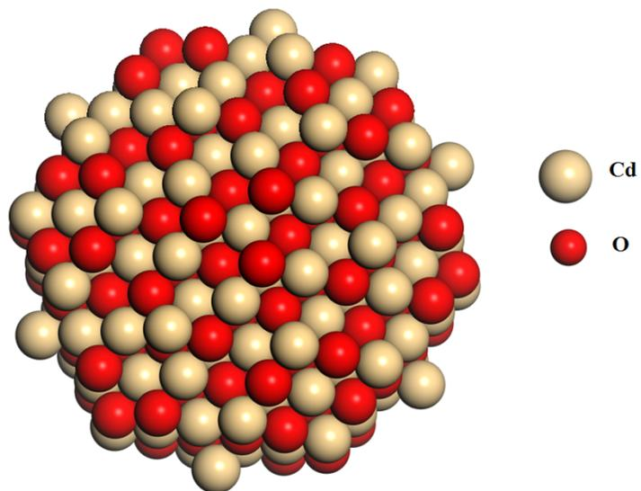
**Figure S2.** CdO nanoparticle, containing 341 atoms constructed by Wulff scheme, and used in DFT calculations.
