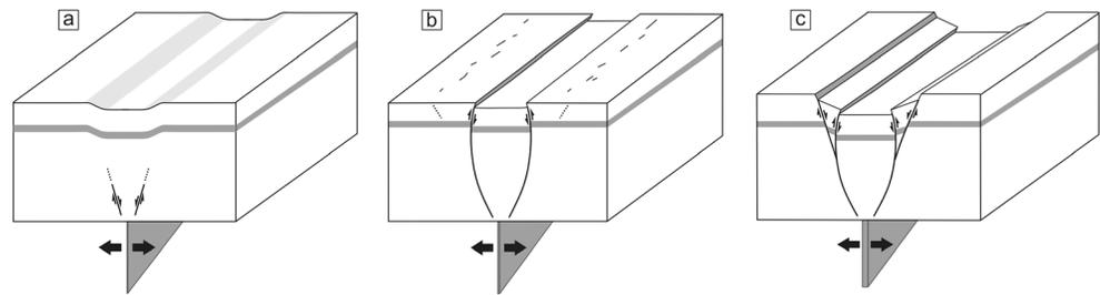
**Figure 4.** Summary of the main stages of surface deformation due to the emplacement of the dikes. (a) Depression at the surface, (b) inner set of arcuate faults propagating upward and reaching the surface as high-angle reverse faults, and (c) outer set of normal faults propagating downward and merging with the inner faults at depth. The tilted blocks lie between the outer and inner faults.
