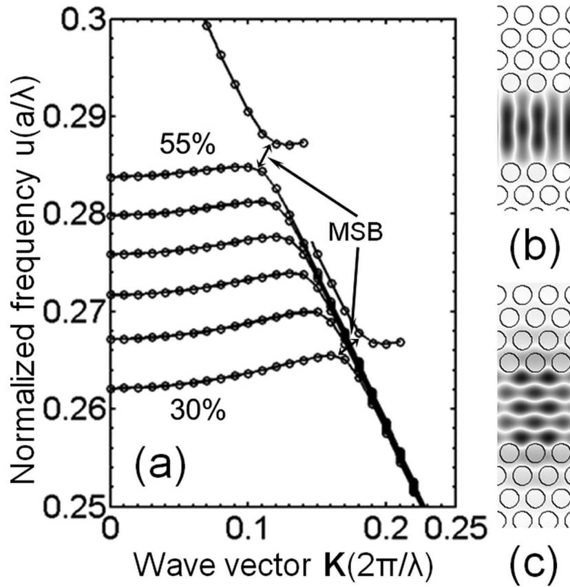
FIG. 1. (a) Dispersion diagram of the W3 Waveguide showing the investigated mode-gap and its evolution with  $f$  which was varied from 30 to 55%. Mode profiles of (b) 0<sup>th</sup> order mode and (c) 4<sup>th</sup> order mode sufficiently far away from the mode-gap region.
