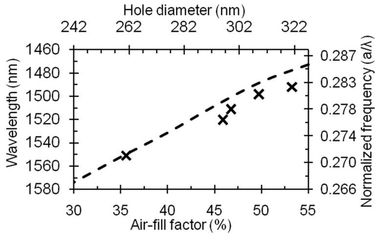
FIG. 2. MSB central frequency vs.  $f$  for W3 PhC waveguide. Secondary axes are scaled with a lattice constant  $a = 420$  nm. The dashed line represents MSB shift obtained by 2D FDTD calculations while the “X” symbols the experimental determined air fill factors central MSB positions.
