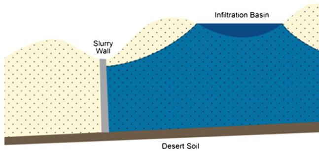
**Figure 4.** Design concept of the dune aquifer stormwater storage system.
