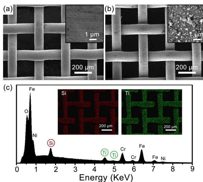
**Figure 1 | Morphology and surface composition of the stainless steel mesh after the LbL assembly of (silicate/TiO<sub>2</sub>)\*20 coating.** SEM images of the original stainless steel mesh (a), and the (silicate/TiO<sub>2</sub>)\*20 coated mesh (b). Insets in (a) and (b) show the magnified view of the knitting wire surfaces. (c) EDS spectrum of the (silicate/TiO<sub>2</sub>)\*20 coated mesh. The insets in (c) show the SEM-EDS elemental mapping of Si and Ti.
