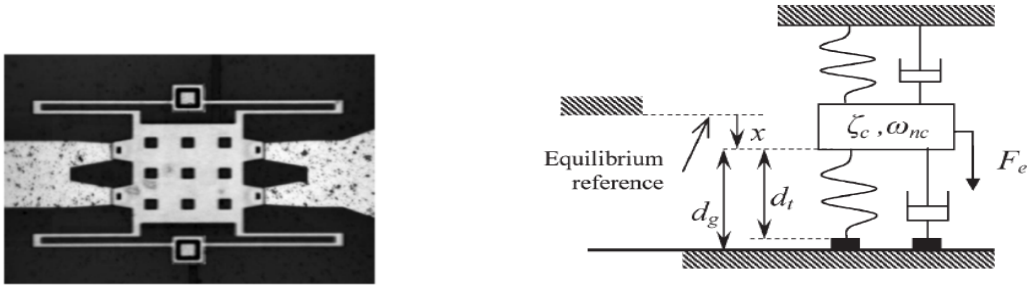
Figure 4: SEM image of RF switch and lumped mass model [5]
