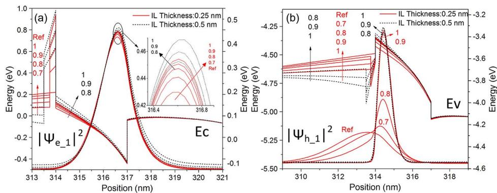
Fig. 5. Band diagram and wavefunction profiles corresponding to a) electron and b) holes, in the active region, for different structures. The fraction indicated, such as 0.7, 0.8, 0.9, and 1 are the Al compositions, and the Ref structure does not have the IL layer. The solid red line and black dotted line represent the insertion layer (IL) thicknesses of 0.25 nm and 0.5 nm, respectively.
