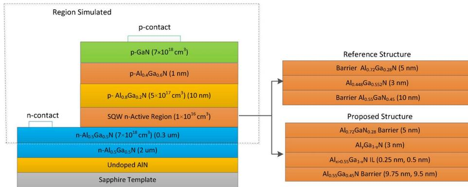
Fig. 1. Schematics of the full UVB LED structure, the reference structure design, and the proposed structure design with thin AlGaN monolayer insertion (MLI).
