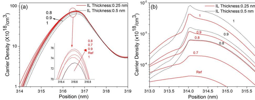
Fig. 2. Carrier densities of (a) electrons and (b) holes, under forward bias of 4.5 V, for insertion layer with different thicknesses and Al mole fraction.
