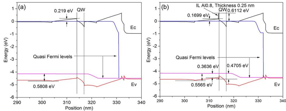
Fig. 4. Band diagram, under forward bias of 4.5V, for structure A and C.
