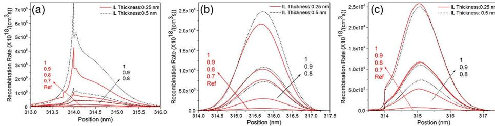
Fig. 3. Recombination rates of: (a) *SRH*, (b) *Auger* and (c) Direct, in the quantum well region (314 nm–317 nm) under forward bias of 4.5 V, for insertion layer with different thicknesses and Al concentrations. The solid red line and black dotted line represent the insertion layer (IL) thicknesses of 0.25 nm and 0.5 nm, respectively.
