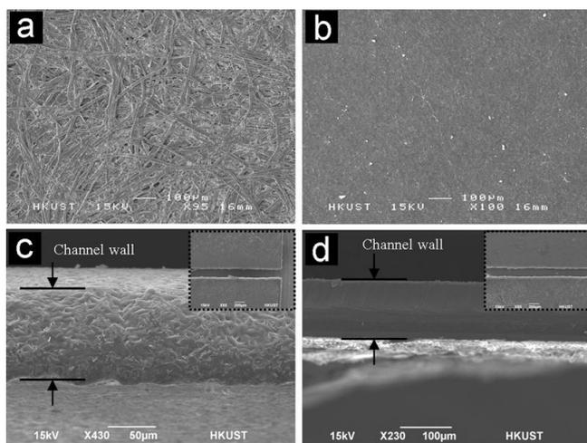
**Fig. 2** (a) Surface morphology of A4 wood paper before absorbing wax, (b) after absorbing wax, (c) channel wall of wax-filled paper. (d) channel wall of transparent film. The inset pictures are the corresponding wax paper and transparent film channels.
