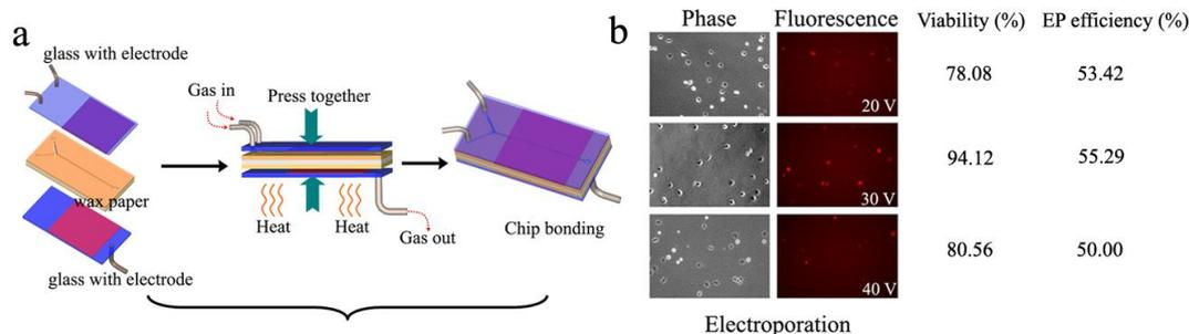
Fig. 4 (a) The flow chart to show the fabricating process of a wax-paper-based microfluidic device with imbedded electrodes. (b) The images of cells under bright field and fluorescent field. The cell viability and the EP efficiency are also presented.
