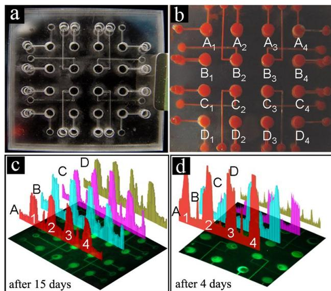
**Fig. 5** (a) Top view of 5-layer 3D structure, (b) Red dye solution was infused to indicate screening chambers, (c) GFP recombinant *E. coli* bacteria were cultured in screening chambers showing green fluorescence protein. The peak appears at the row A, B, C, and D labeled by digits 1, 2, 3, and 4 is to show the intensity of fluorescence corresponding to the screening chamber beneath them, (d) The chemotaxis phenomenon of *E. coli* bacteria responding to the antibiotic concentration.
