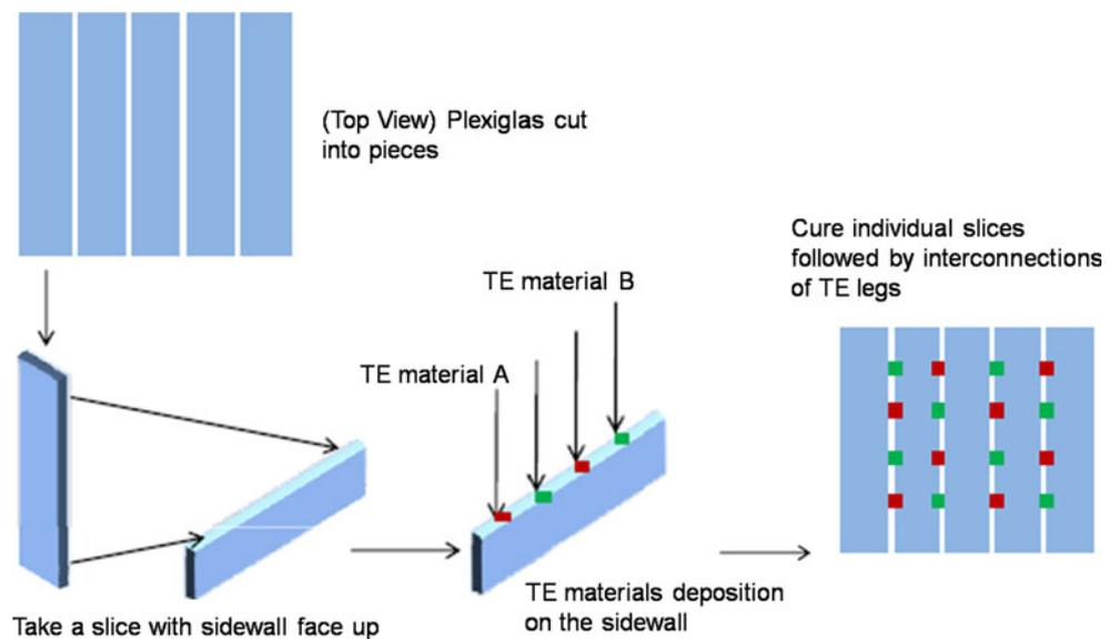
**Fig. 3** 3-D Schematic of the checkerboard device. *Inset* shows original checkerboard TE slide
