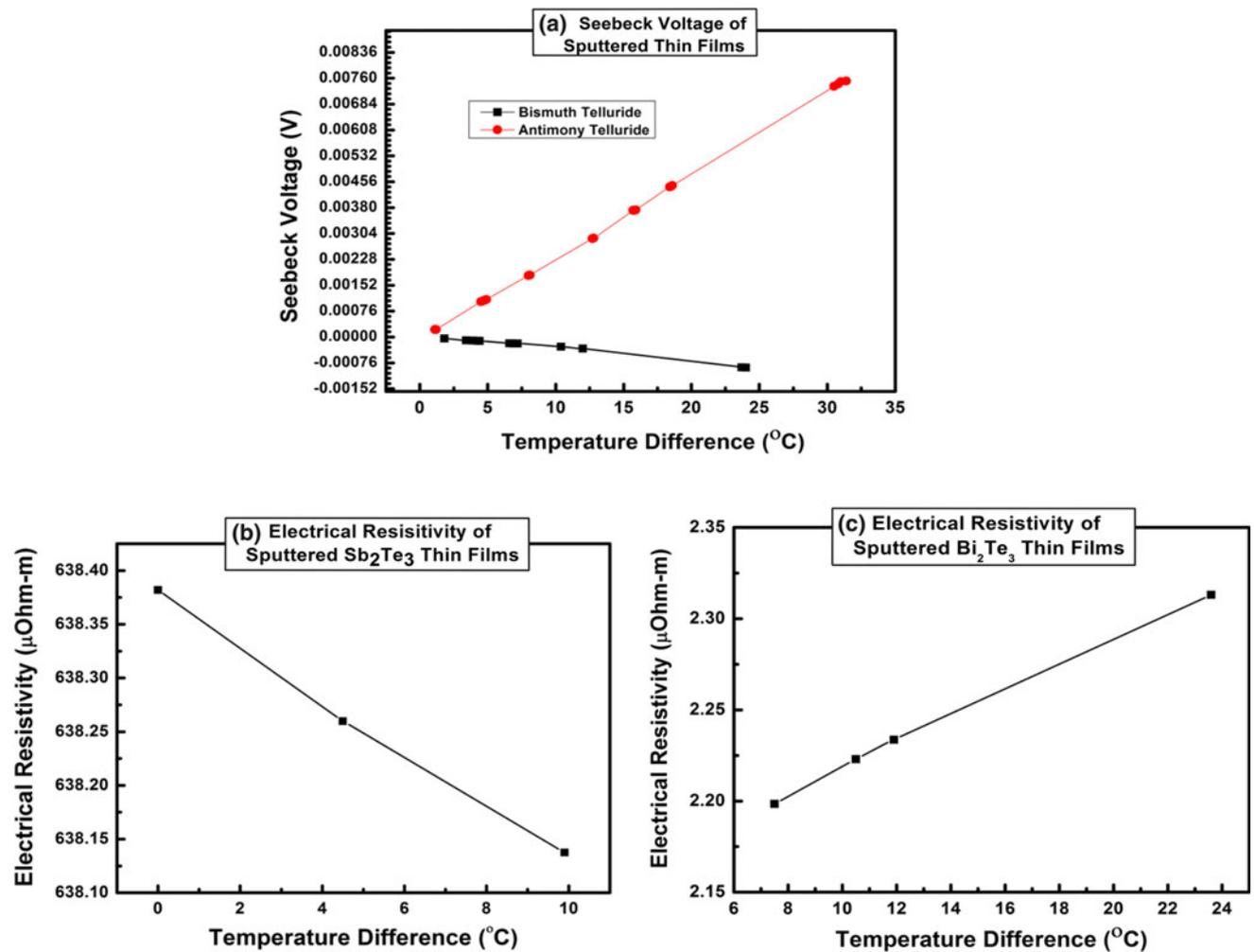
**Fig. 8** Thermoelectric properties of sputtered thin films: **a** Seebeck coefficient of Sb<sub>2</sub>Te<sub>3</sub> and Bi<sub>2</sub>Te<sub>3</sub>, **b** electrical resistivity of Sb<sub>2</sub>Te<sub>3</sub>, **c** electrical resistivity of Bi<sub>2</sub>Te<sub>3</sub>
